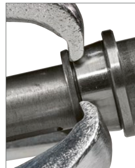
軸上為錐形滾柱軸承
