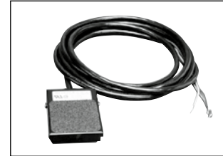
251660 – Foot switch with 3,1 m cord. Single pole, double throw, 15 amp @ 125-250V. Wt., 0,5 kg.
